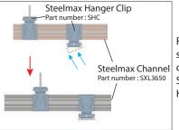
Fixing of secondary channel to Steelmax Hanger Clip
