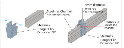
Fixing of Steelmax Hanger Clip and SteelMax Channel SXL3650
