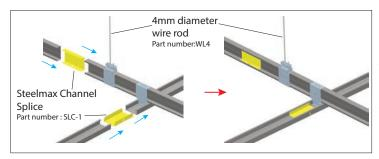
Fixing of Steelmax Channel Splice SLC-1 and SteelMax Channel SXL3650
