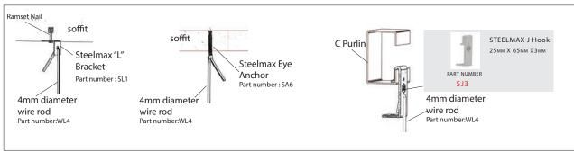
Roof purlin, soffit of slab suspension details
