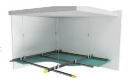
diameter which are connecting to SteelMax Butterfly Spring Clip"BSC" (BMT 0.58mm) and Suspension Galvanized Wire Rod 4mm in diameter fixed onto the soffit using "Eye anchor" at 1200mm centres; Board edges at perimeter is fixed onto SteelMax Perimeter "SLP2440" (BMT 0.5mm). All boards joints secure with Gyproc or AGP Paper Tape and finished with Protop Joint Compound for a seamless finish. All fixing accessories, additional nogging for services installation as per manufacturer details
