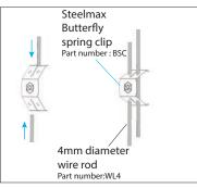
Connecting 4mm diameter wire rod to Butterfly spring clip
