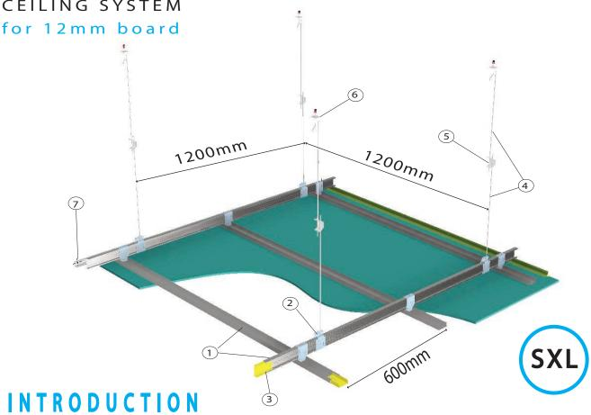
The SteelMax SXL ceiling system is a carefully engineered metal framing structure suitable for suspended concealed ceiling construction to be lined with a wide range of ceiling lining materials i.e. gypsum plaster-board, calcium silicate or fibre-reinforced cement panels, etc. When constructing according to recommended specifications, the ceiling system is designed to meet the most sought after functional features nowadays such
