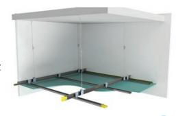
diameter which are connecting to SteelMax Butterfly Spring Clip"BSC" (BMT 0.58mm) and Suspension Galvanized Wire Rod 4mm in diameter fixed onto the soffit using "Eye anchor" at 1200mm centres; Board edges at perimeter is fixed onto SteelMax Perimeter "SLP2440" (BMT 0.5mm). All boards joints secure with Gyproc or AGP Paper Tape and finished with Protop Joint Compound for a seamless finish. All fixing accessories, additional nogging for services installation as per manufacturer details
